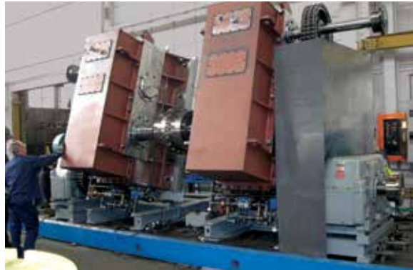
Photos show Nuttall's massive in-house custom-built test stand with two of the 15,000 lb. Fort Street bridge reducers mounted and being tested on a 75-degree incline per specification.
